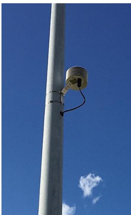
Figure 4-6. An ‘eNose’ on a lamppost at the Moerdijk port and industrial park.
